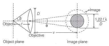
Here, limit of resolution of microscope  $d = \frac{1.22f\lambda}{D}$
